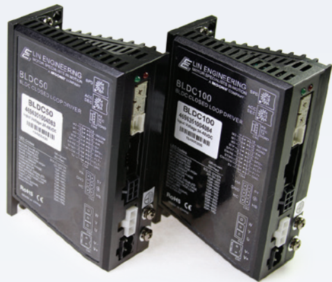
◀ BLDC50/100 BLDC Driver/Controller • 12-48 VDC supply voltage • Work in velocity mode • Accept analog control signal, digital control signal, RS-232/485 communication command, or MMI control.
