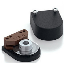
E2 ENCODER Features and Benefits: • Best for NEMA 17, 23, and 34 • 32 to 5,000 cycles per revolution (CPR) • Tracks from 0 to 300,000 cycles/sec • 128 to 5,000 pulses per revolution (PPR)
