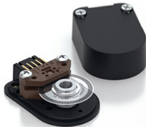
E5 ENCODER Features and Benefits: • Best for NEMA 23 and 34 • 32 to 5,000 cycles per revolution (CPR) • 128 to 5,000 pulses per revolution (PPR) • Tracks from 0 to 100,000 cycles/sec
