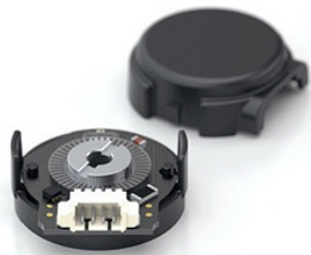
E4T ENCODER Features and Benefits: • Compact miniature size best for NEMA 8, 11, 14, and 17 • 100 to 500 cycles per revolution (CPR) • Tracks from 0 to 100,000 cycles/sec • 400 to 2,000 pulses per revolution (PPR)
